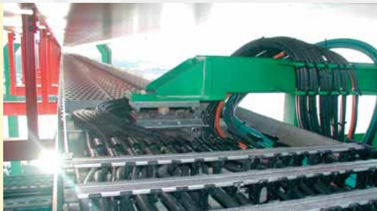
Energy guiding chain designed for long travel distance on a ship-to-shore container crane
