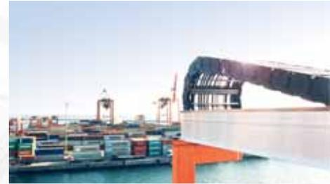
Cobra energy guiding chain installed on a stacking crane
