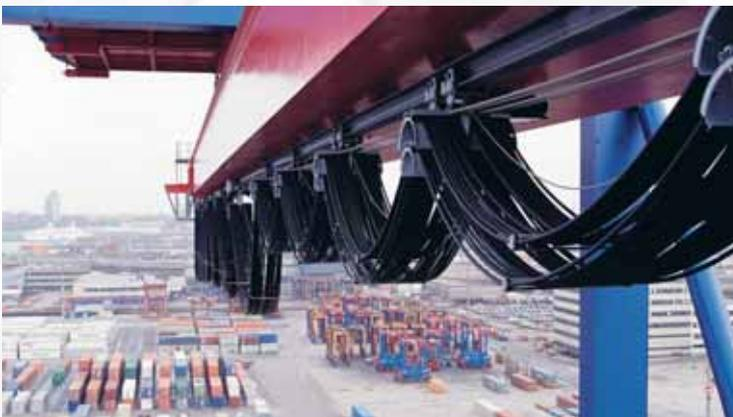
Motorized cable trolley system on a ship-to-shore container crane
