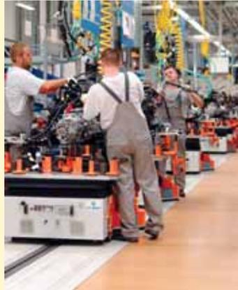
Unlike power transfer systems that use mechanical contacts or components, IPT®-Rail functions completely without contact. As a result, there are no mechanical parts that can wear out or limitations in terms of travel speed or acceleration. Since wear is completely eliminated, IPT® is especially recommended for use in environments that call for special requirements with respect to cleanliness or hygiene.
