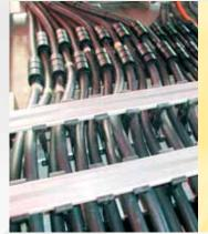
Cable for energy guiding chains with clips for strain relief
